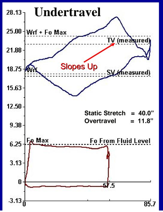
**Undertravel** Surface card slopes upward from left to right. The pump plunger moves *less* than the plunger stroke. Undertravel is due to rod stretch from fluid load, downhole friction or other reasons. Undertravel cards include: stuck pumps, *plunger is too large for the rod string*, sand or scale problems, too tight stuffing box and/or paraffin.
