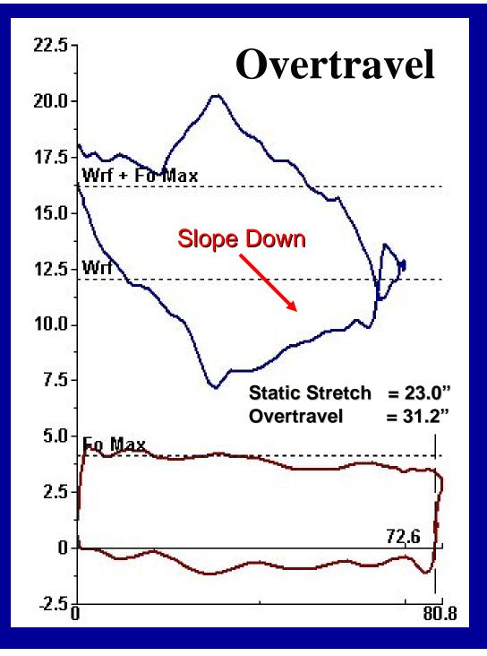
**Overtravel** Plunger stroke is longer than PR stroke. Surface card slopes downward from left to right. Example: The 80.8" plunger stroke is *more* than the 72.6" polished rod stroke. The surface stroke is reduced by 23" of rod stretch required to lift the fluid load. The 13.74 SPM adds momentum to the rods increasing stroke by 31.2" inches. Overtravel cards include: parted rods, flowing wells, unseated pumps, gas locks, worn pumps, fiberglass rod strings or pumping at a very fast SPM.
