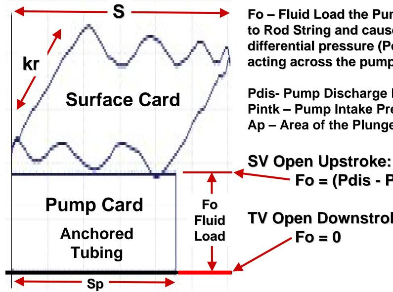
**Fo – Fluid Load the Pump Applies** to Rod String and caused by the differential pressure (Pdis-Pintk) acting across the pump plunger.
